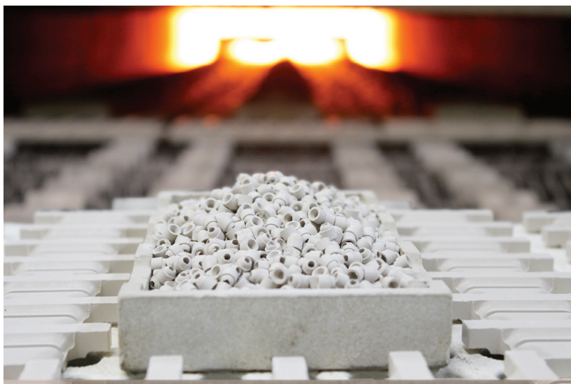
A view of some of the Steatite components lined up in front of the Ceramicx kiln
