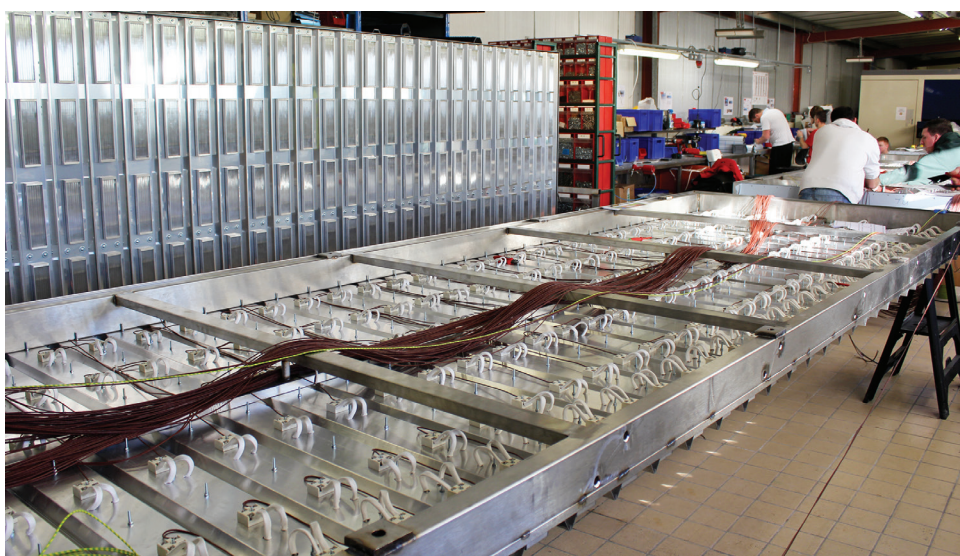
An image of the IR platens under construction at Ceramicx
